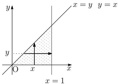
$$\begin{aligned} & \int_0^1 \left\{ \int_y^1 e^{-x^2} dx \right\} dy = \iint_D e^{-x^2} dx dy \\ &= \int_0^1 \left\{ \int_0^x e^{-x^2} dy \right\} dx = \int_0^1 \left[ ye^{-x^2} \right]_{y=0}^{y=x} dx \\ & \quad \text{\color{red}x は定数扱い} \\ &= \int_0^1 xe^{-x^2} dx = -\frac{1}{2} \int_0^1 (-x^2)' e^{-x^2} dx \\ &= -\frac{1}{2} [e^{-x^2}]_0^1 = -\frac{1}{2} (e^{-1} - 1) = \frac{1}{2} \left( 1 - \frac{1}{e} \right) \end{aligned}$$
