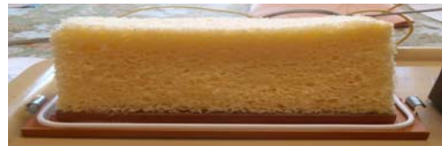
Fig.12 "Electrode cake" with whole egg whipped batter energized.
