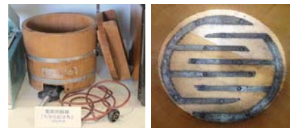
Fig.7. (Left) "comb-teeth" type rice cooker called "Takara-Ohachi" (from the collection of the Osaka City Museum) (Right) comb teeth shaped plate at the bottom of the container(released around 1947).
