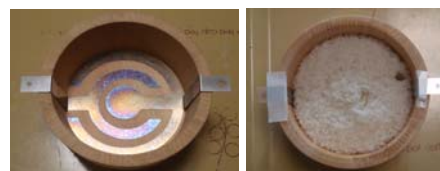
Fig.9. (Left) Concentric rice cooker with a bottom-mounted rice container (reproduction of "welfare type" made by myself) (Right) Cooked rice: in 20 minutes.
