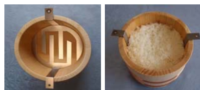
Fig.8. (Left) Rice cooker with bottom-mounted comb-teeth in the shape of a rice container (reproduction of "Takara-Ohachi" made by myself) (Right) Cooked rice: in 25 minutes.
