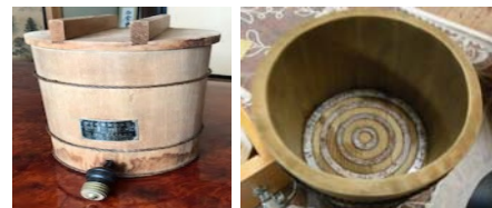
Fig.6. (Left) "welfare type" rice cooker(from the collection of Hiratsuka City Museum) (Right) Concentric circular plate at the bottom of the container.
